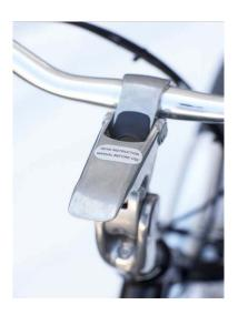
Push up the black button and raise the lever to allow for adjustment of the handlebars in desired position.
