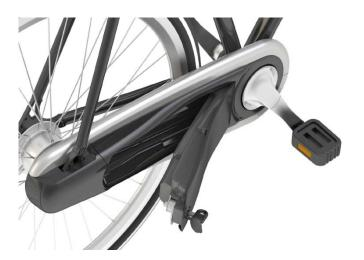
The battery is integrated in the bicycle chain case.
